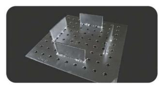
The sump cover will fit the manhole sump and shall not rock when installed. The sump cover shall be manufactured from a square steel plate, thickness of the steel is approximately 5mm with 10mm diameter holes and It will be capable to support a point load of ≥100Kg.
