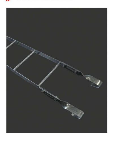
Provides a secure and easy entry into and exit from the manhole. The ladder rungs will be non-slip corrugated steel bars 16mm in diameter, welded to a pair of ladder rails. Each ladder rail will be fitted with a hook, securely fixed to the inner part of the side rails with bolts, lock washers and nuts.
