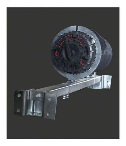
The Swiveling telescopic closure bracket for fastening to the handhole wall as a metallic holder. Swivel arm and bracket shall be manufactured from 4mm thick steel and Hot dip galvanized finish. The structure has to hold a fiber access terminal type of closure distributing the drop cable along with their drop duct and it will be able to load bearing approx. 250 N.
