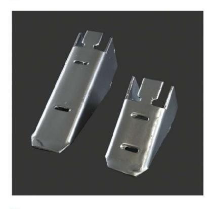
Cable Bracket shall be manufactured from approximately 4 mm thick steel, with capacity for Vertical load ≥ 1.5 kN and Horizontal load ≥1 kN, Cable bracket that is horizontally fixed at one end only and spaced at specified intervals along the manhole walls to support cables and cable joints.
